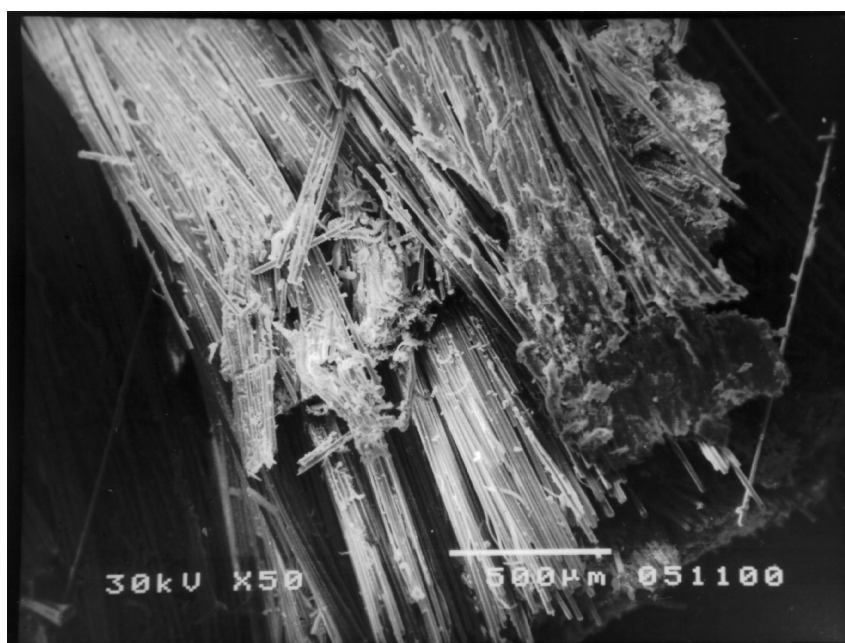
Figure 8. Fracture surface micrograph of the impacted specimen ( \times 50 ).
